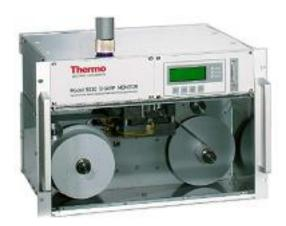
Quick and reliable, the SHARP PM monitor with TUEV approval according to the European Norms for PM10 and PM2.5 monitoring.
