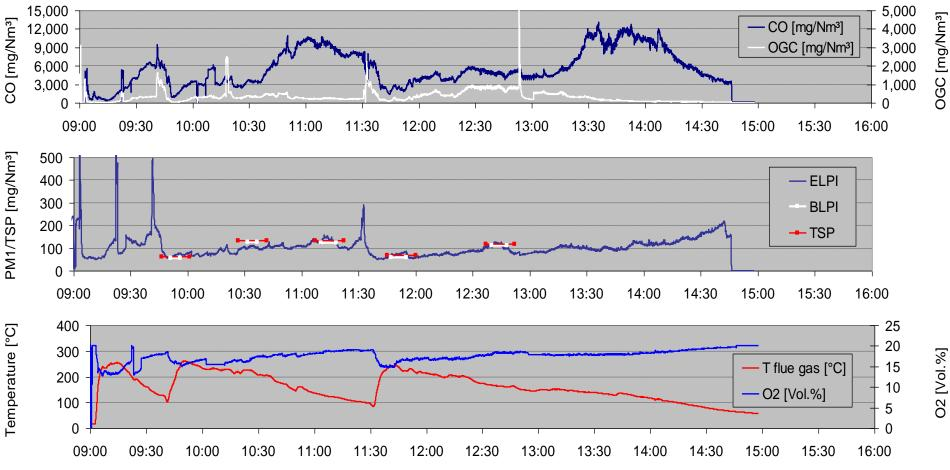
Emissions related to dry flue gas and 13 vol% O<sub>2</sub>, TSP ... total suspended particulate matter, ELPI ... PM<sub>1</sub> emissions by electrical low pressure impactor, BLPI ... PM<sub>1</sub> emissions by Berner-type gravimetric low pressure impactor
