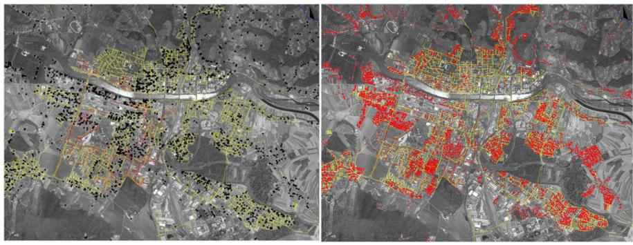
Spatial distribution of combustion plants together with gas piping (yellow lines) and hot-water piping (red lines) networks in the municipality
